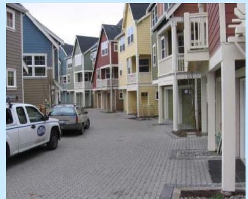
Stormwater drains through this permeable paver drive to a stone storage layer.
